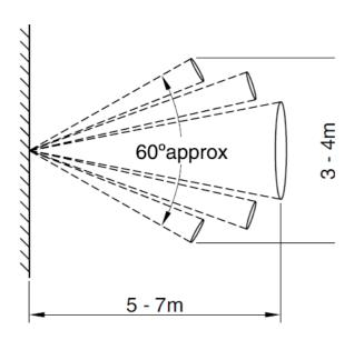
The elliptical beam gives 360° detection with a Plan view arc of 100° and Side view arc of 60° and detects infra-red body heat passing or approaching the sensor.
